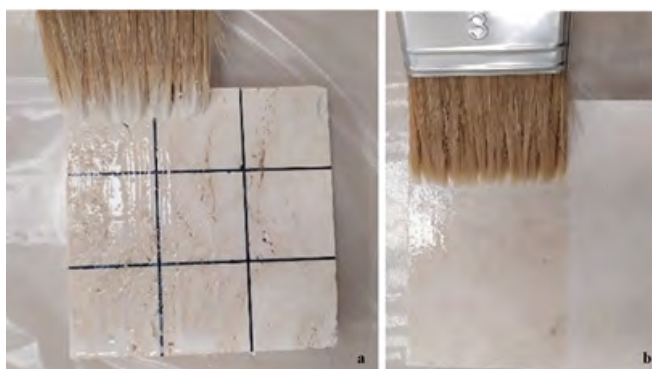
Fig. 3. Water-repellent chemical application process a) water-based water-repellent chemical application, b) solvent-based water-repellent chemical application
